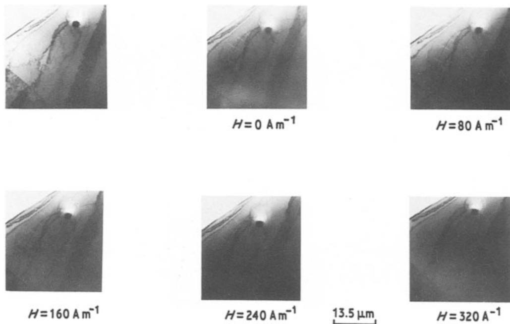
Figure 3 Pinning effect of domain walls by a particle and a grain boundary.
