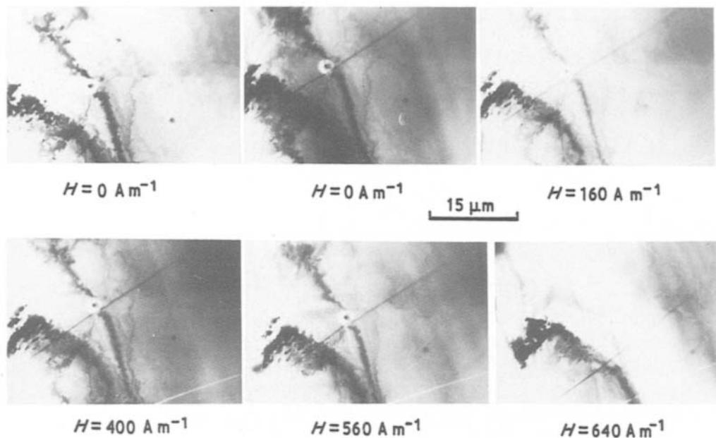
Figure 1 Interaction of black and white walls in a thin ferromagnetic film.
