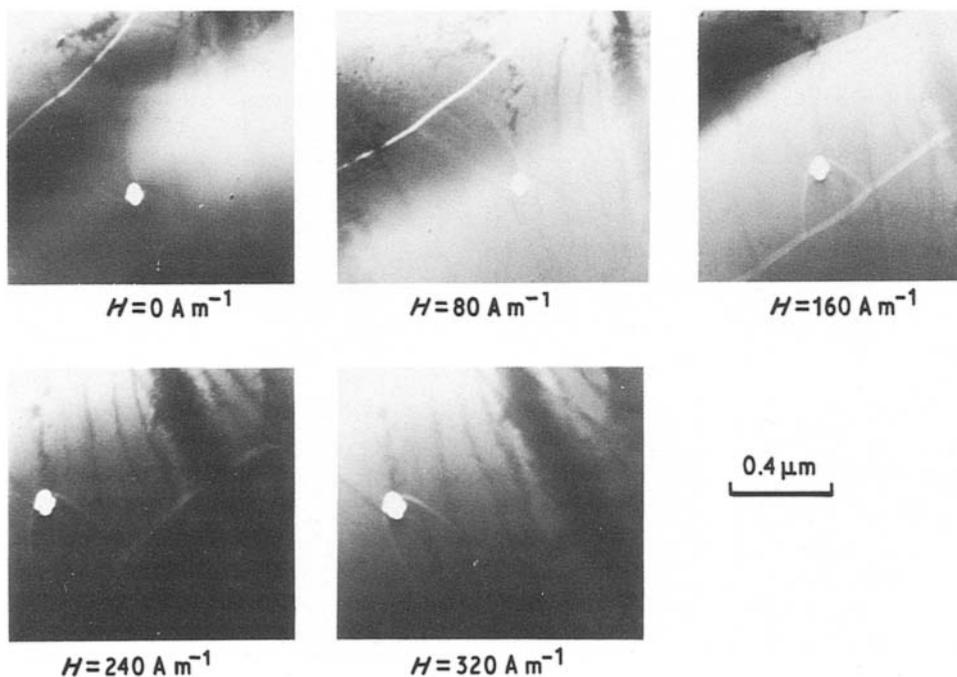
Figure 5 Pinning of domain wall by an inclusion (note the parabolic wall formed around the inclusion in order to reduce magnetostatic energy of the wall).
