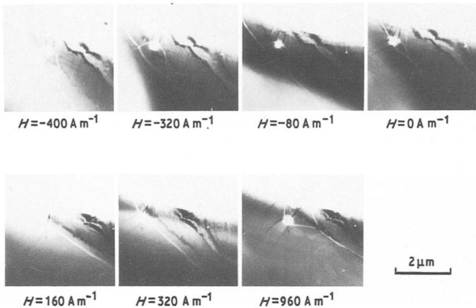
Figure 4 Pinning of domain walls by two holes.
